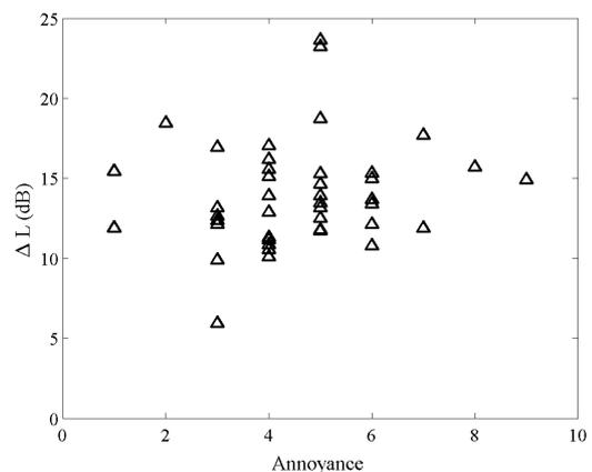
Figure 8. Amplitude modulation depth versus resident rated Annoyance level.
